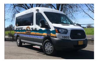
RVTD added six hybridelectric passenger vans to its paratransit fleet, decreasing CO<sub>2</sub> emissions by 20% and achieving an increase of 25 mpg over its conventional vans.
