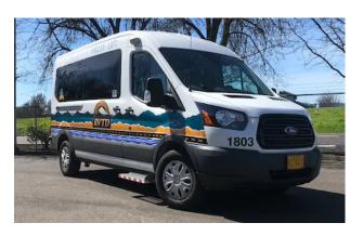
RVTD added six hybridelectric passenger vans to its paratransit fleet, decreasing  $CO_2$  emissions by 20% and achieving an increase of 25 mpg over its conventional vans.
